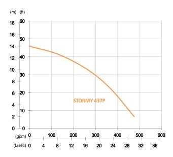
Shaft Speed: 1750 rpm Outlet: 100mm, 4in
